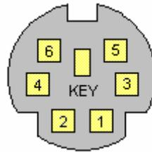
**Figure 5-6.** Keyboard or Pointing Device Interface Connector
