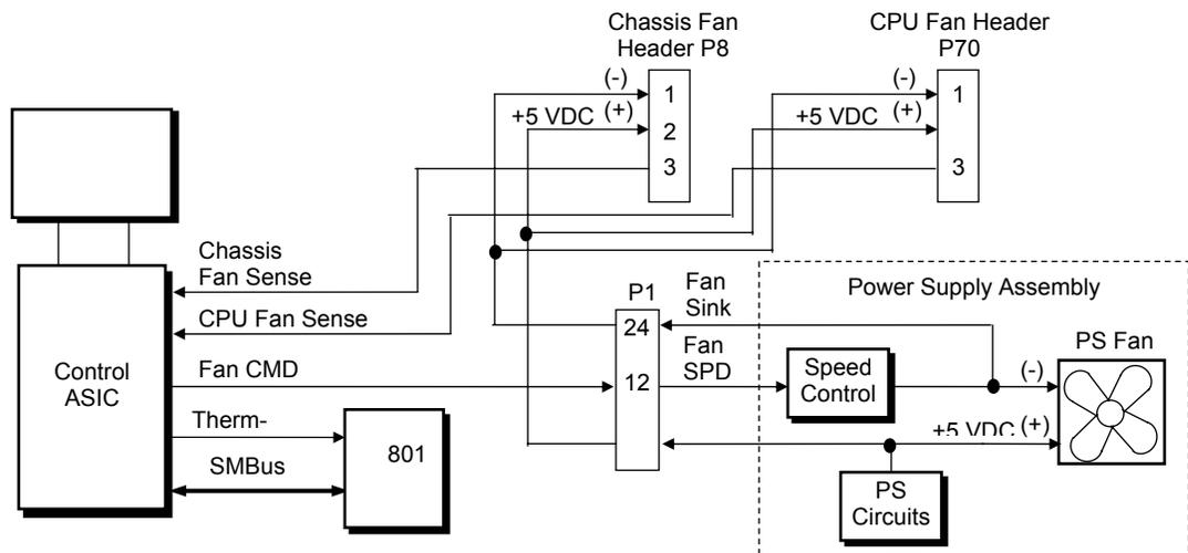
Figure 4-12. Desktop/Configurable Minitower Fan Control Block Diagram
