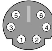
Figure C-9. PS/2 Keyboard Cable Connector (Male)
