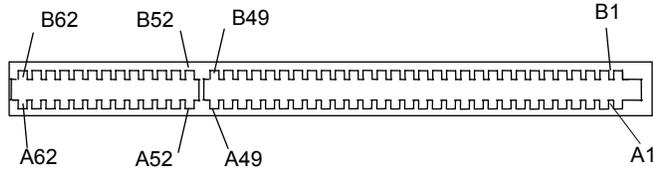
Figure 4-4. PCI Bus Connector (32-Bit Type)
