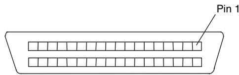
Figure G-3. External Ultra SCSI Connector (50-pin)
