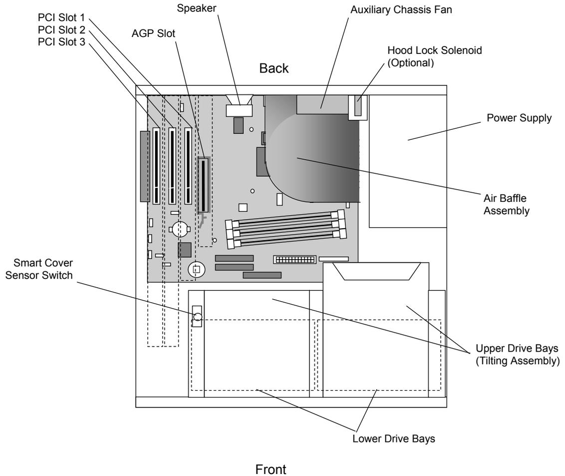
**Figure 2-5.** Desktop Chassis Layout, Top View
