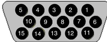
**Figure H-5.** Analog (VGA) Monitor Connector (One of two female DB-15 connectors).
