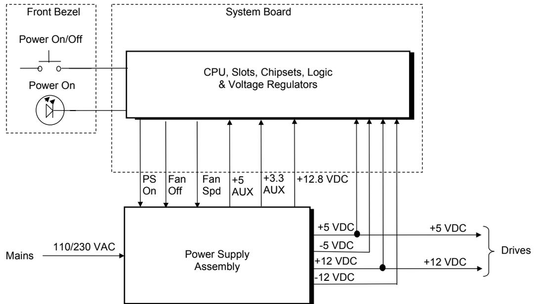
Figure 6-1. Power Distribution and Control, Block Diagram
