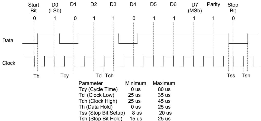
Figure 5-5. 8042-To-Keyboard Transmission of Code EDh, Timing Diagram
