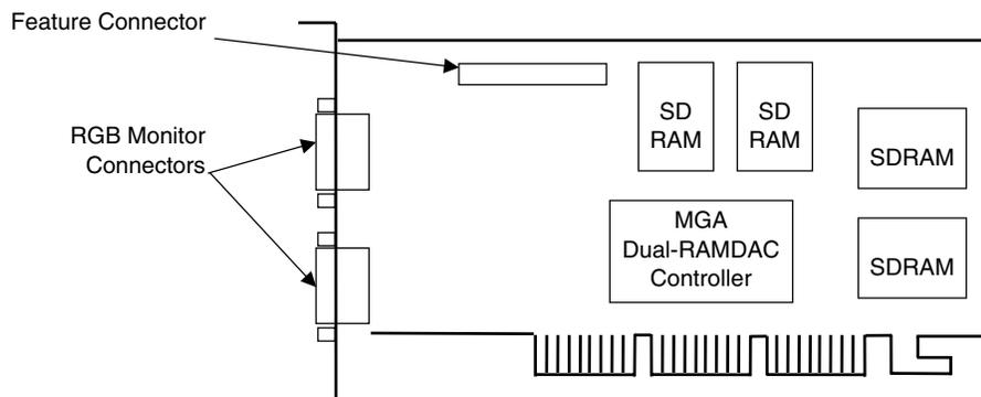
**Figure F-1.** Compaq/Matrox Millennium G450 AGP Graphics Card Layout (PCA# 202901-001)
