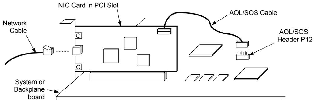
**Figure 5-15.** Remote System Alert Implementation (Generic Representation)
