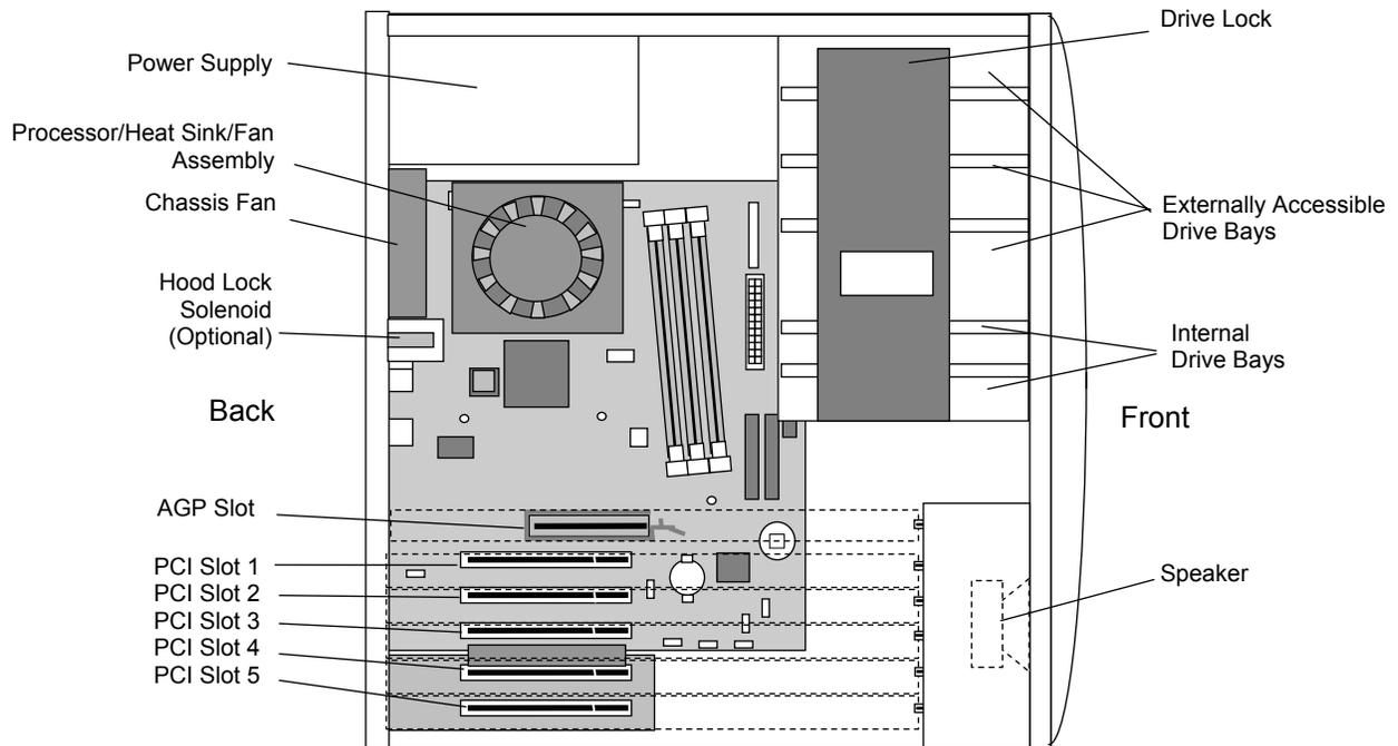
**Figure 2-6.** Configurable Minitower Chassis Layout, Left Side View (Minitower configuration)
