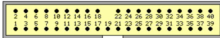
Figure 5-1. 40-Pin Primary IDE Connector (on system board).
