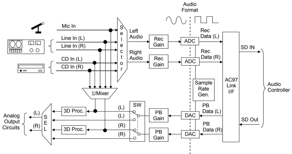
**Figure 5-12.** AD1885 Audio Codec Functional Block Diagram
