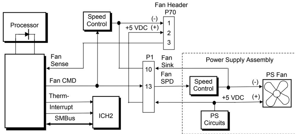
Figure 4-11. Small Form Factor Fan Control Block Diagram
