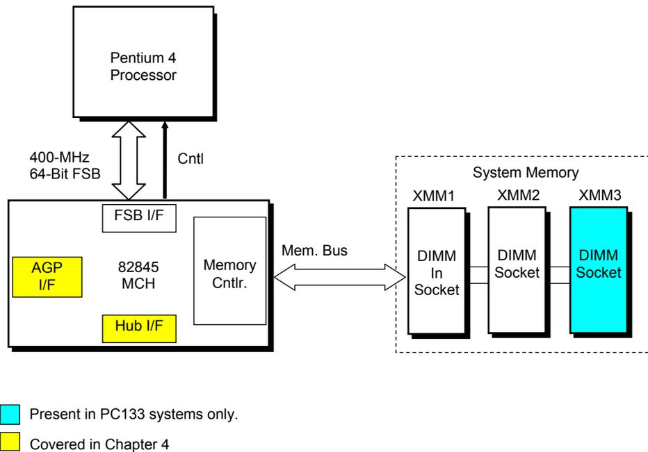
**Figure 3-1.** Processor/Memory Subsystem Architecture
